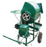
Figure 12: Field testing of portable paddy thresher
